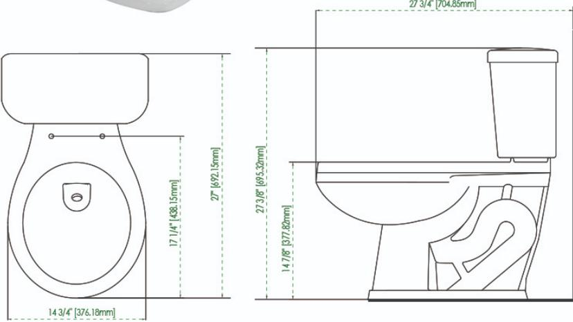
Dimensions: 14 3/4" [376.18mm] x 17 1/4" [438.15mm] x 27" [692.15mm] (front view); 14 7/8" [377.82mm] x 27 3/8" [695.20mm] x 27 3/4" [704.85mm] (side view).
